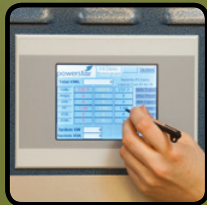
The Powerstar Human - Machine Interface (HMI) shows every detail of the site electricity supply in real time.
